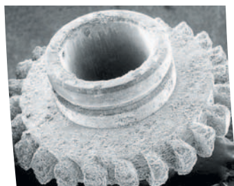
Handpiece serviced with a common lubricant.
